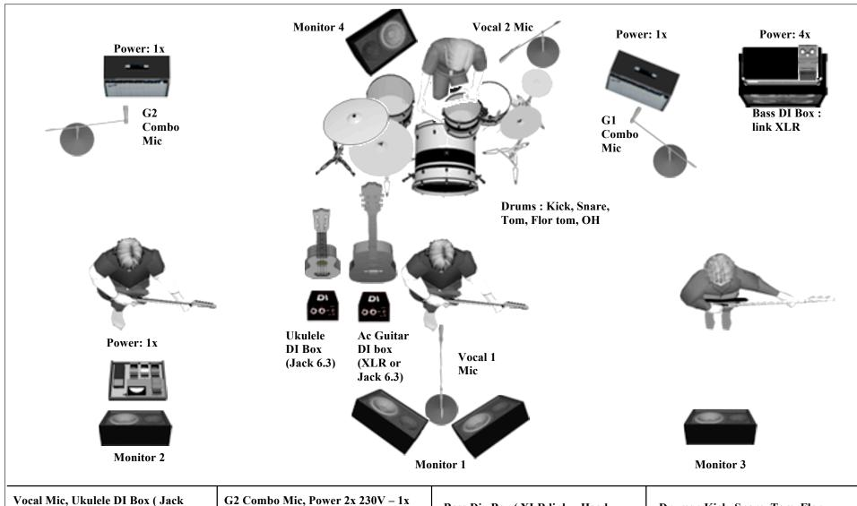
Vocal Mic, Ukulele DI Box ( Jack 6.3), Acustic G (DI Box XLR or Jack), G1 Electric Combo (Mic), 1 x Power 230V
